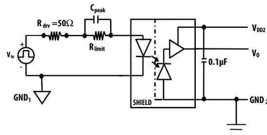
Figure 10. Connection of peaking capacitor ( $C_{peak}$ ) in parallel of the input limiting resistor ( $R_{limit}$ ) to improve speed performance
