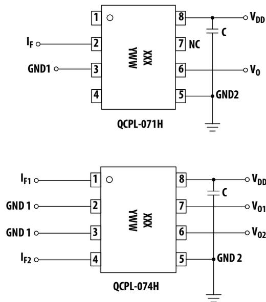
$C = 0.01\mu\text{F}$  to  $0.1\mu\text{F}$
