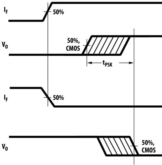
Figure 8. Propagation delay and skew waveform
